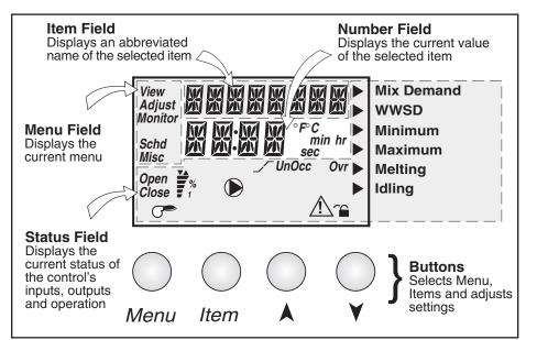
The tekmar Mixing Control 362 has a Liquid Crystal Display (LCD) and four push buttons (*Menu*, *Item*, A, $\forall$ ) which are used to view and adjust the settings.
